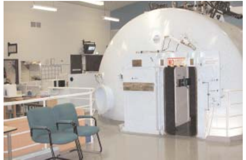
A recompression chamber: the only definitive treatment for decompression.
